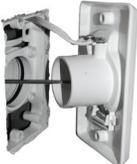
Pass a piece of bent coat hanger into the inlet then into the mounting plate. Holding the mounting plate with the bent coat hanger, install the inlet using the screws provided in the installation kit. Do not cement the inlet - a sealing gasket is already installed in the mounting plate. If the screw at the level of the pipe is too long and could pierce the pipe, use the shorter screw provided with the installation inlet.
