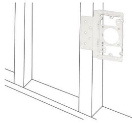
Install piping before partitions are enclosed. The mounting plate can be attached directly adjacent to the studs using its installation support.
