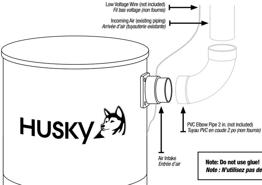
④ LOW VOLTAGE WIRE CONNECTION | RACCORDEMENT DES FILS BAS VOLTAGE
